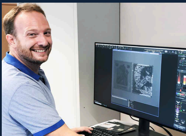
Tobias Huylmans uses the spectral analysis function of the VSC 8000 to present an authentic China handstamp (right) and a forged one (left).
